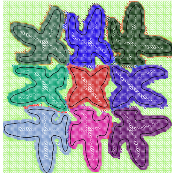
Fig. 2. Example of extending the orientation angle in the liquid phase. The orientation angle is extended to the liquid phase with \phi < 3w . The artifacts of interpolation lead to a color different from all nearby colors at some places of the mesh. The plotting software we utilized, Tecplot [31], automatically interpolates the orientation and plots the color corresponding to the interpolated value.
